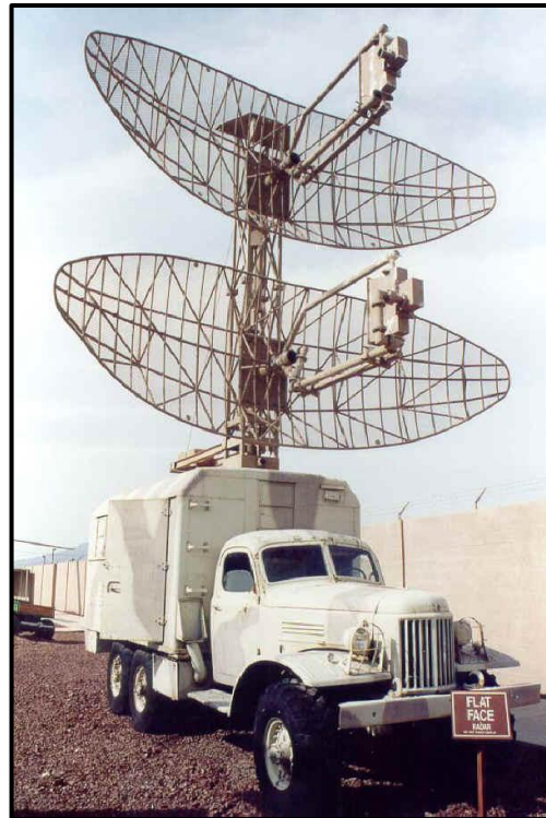
Above left is a typical Neva SAM site, above right is the P-15 Flat Face target acquisition (EW) radar.
