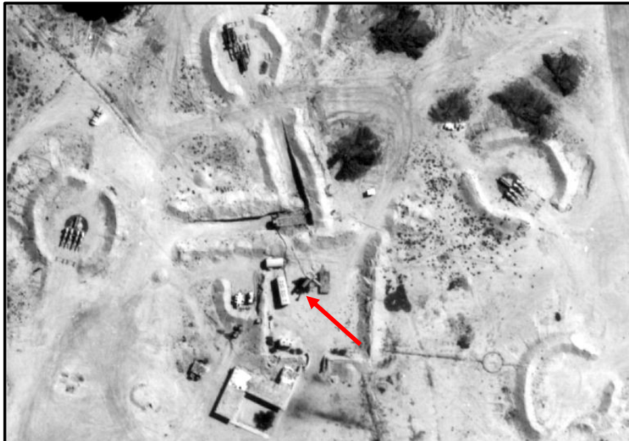
Above is a Neva battery in Middle East. The battery had only 3 missiles rails – very likely one destroyed previously – in the middle are the SNR-125 UNV and UNK cabins (red arrow.)
