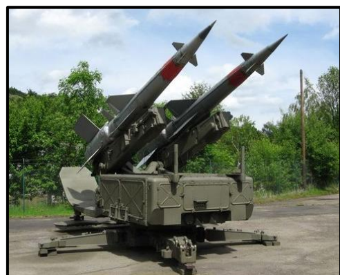
Above left is the quadruple 5P73 launch rail; on right is the dual 5P71 launch rail.
